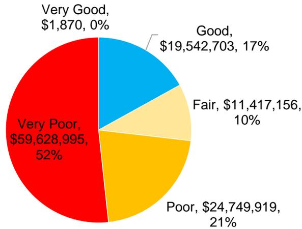
The figure below provides further detail on the water network, by asset type. Based on age, the vast majority of water distribution assets, including mains and service leads, are in poor or worse condition. Although the treatment plant is, based only on age, in good condition, the facility is not componentized; as such, the age of individual facility elements is not known. As such, their condition cannot be approximated.
