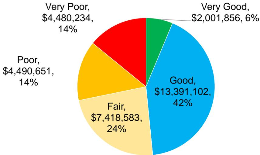
The figure below provides further detail on the road network, by asset type. Based on recent condition assessments, the majority, 60% of roads are in good to very good condition.
