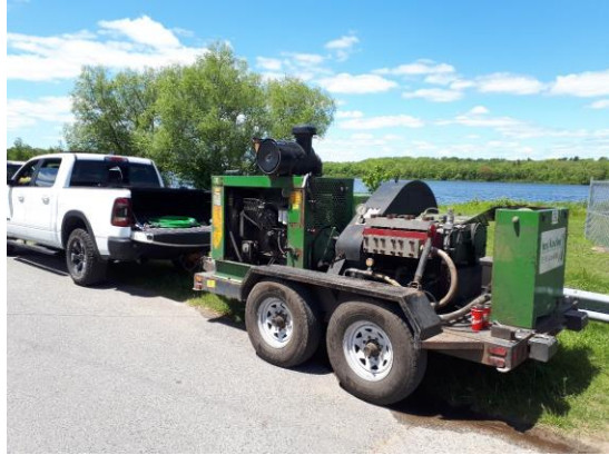
Photo 4: High Pressure Jetting Pump
