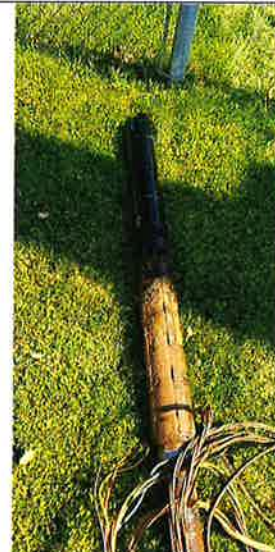
Photo 6: Fouling on Pump
